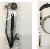
Test fit rudder control horn and pull-pull cable, then glue the control horn in position. Put clevis on control horn side and turn buckle on servo side. Once the pull-pull system is installed, use turn buckles for adjustment. Test fit then install taill wheel T-bar linkage with rudder.
