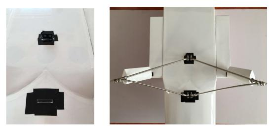
Check your installation and test the suspension cylinder. When you are happy with everything, drip thin CA on the ends of each nut for extra security.
