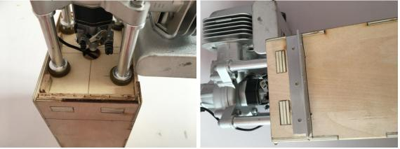
If necessary, trim the openning of dummy engine for engine hub and shaft.
