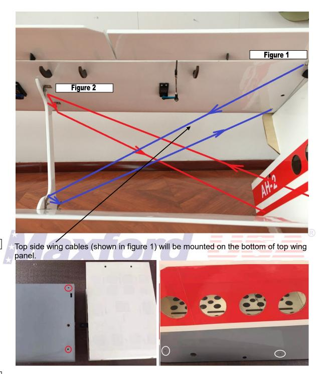
Bottom side cables (Shown in figure 2) will be mounted on the side of fuselage. Use turn buckles on fuselage side for easy disassembly.
