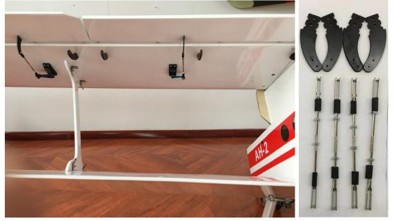
Slide top and bottom wing rods in place, then test fit the left and right wing sets to the fuselage.
