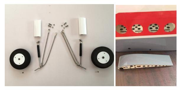
Assemble lower part of landing gear left and right, test fit wheels with self-locking nuts. Slide the white covering piece down to cover the suspension cylinder.
