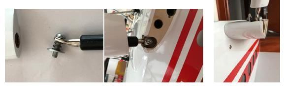
Test fit, and then glue the landing gear mounting tabs into the bottom of fuselage. Test fit, then mount the whole landing gear assemble to the fuselage.
