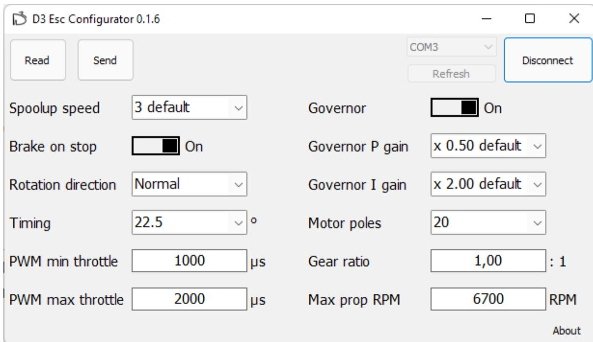
Spoolup speed – this setting change speed of motor reaction for new throttle position. Please remember, fastest setting may overstress drive with abrupt accelerating and braking.
