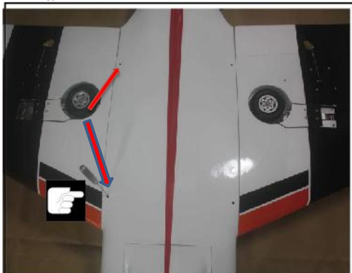
40. Put the fin bolt into the vertical fin.
