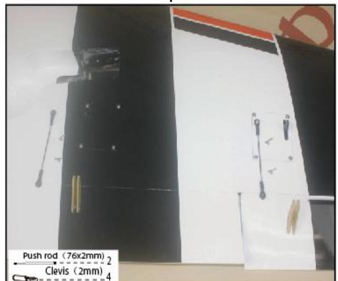
6. Connect the horn to the servo arm with screw.
