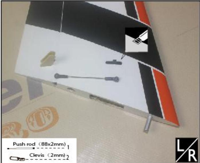
14. Apply instand type AB glue to the slots in the rudder, vertical fin.
