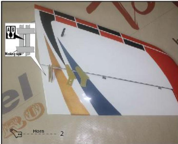
18. Measure the depth to confirm what the servo position will be and open a small slot for the servo arm.
