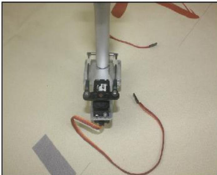
23. Assemble the steering linkages.
