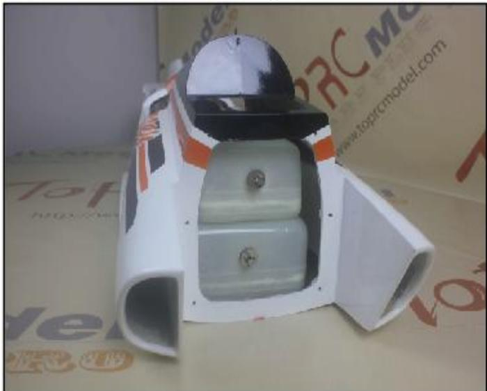
28. Put the tail pipe to the fuselage.
