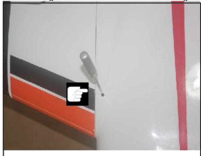
41. Put the vertical fin to the fuselage.
