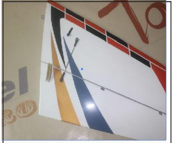
20. Connect the fiber horns to the servo arms with the linkage and locked each side with screws.
