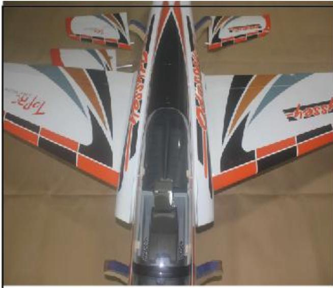
37. Fix the wing to fuselage with screws from the bottom of the wing.
