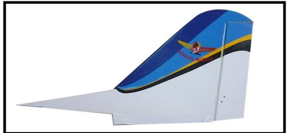
1) Using a modeling knife, remove the covering from over the precut hinge slot cut into the lower rear portion of the fuselage. This slot accepts the lower rudder hinge.
