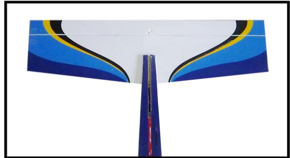
4) With the stabilizer held firmly in place, use a pen and draw lines onto the stabilizer where it and the fuselage sides meet. Do this on both the right and left sides and top and bottom of the stabilizer.
