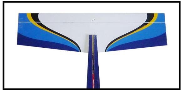
10) After the epoxy has fully cured, remove the masking tape or T-pins used to hold the stabilizer in place. Carefully inspect the glue joints. Use more epoxy to fill in any gaps that may exist that were not filled previously and clean up the excess using a paper towel and rubbing alcohol.
