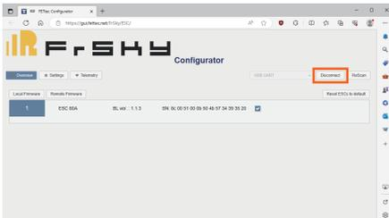
Step 3: Connect the NEURON2 ESC to the S.Port 2 and switch the Dip to "Upgrade" mode. Once powering the ESC then, please click the "Connect" button in 5 seconds to complete the connection.
