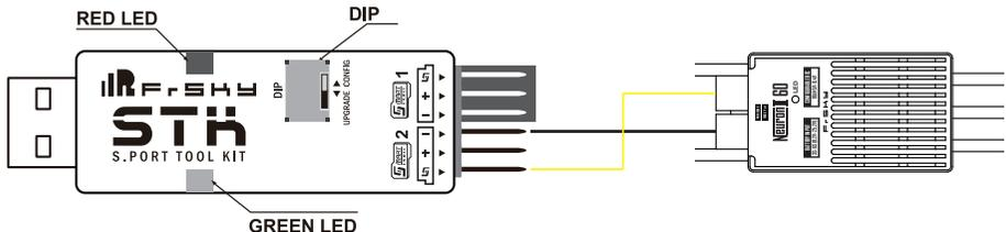
**Note: To configure the Neuron II ESC, please connect the STK tool to your computer and connect the power supply to the Neuron II ESC. Once powering the ESC then, please click the "Connect" button on Webpage Configurator in 5 seconds to complete the connection.**
