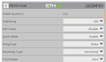
**Note: The settings for Stable System 1 and 2 are independent, and both need to be calibrated when Self Check calibration is required.**
