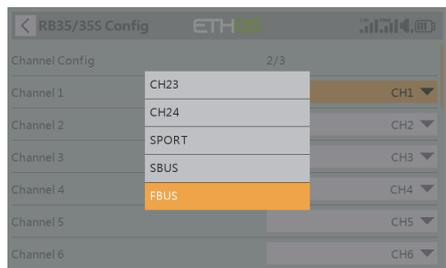
Select the FBUS/S.Port/SBUS for the channel ports.
