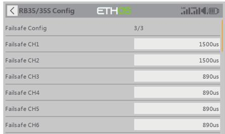
The programmed channel will output the setted Failsafe value before losing the control link.
