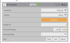
For TW Mode as an example, select the Set [Register] for getting the radio into Registration status in the RF System-Internal Module tool, then press the F/S button on the receiver and power the receiver on.
