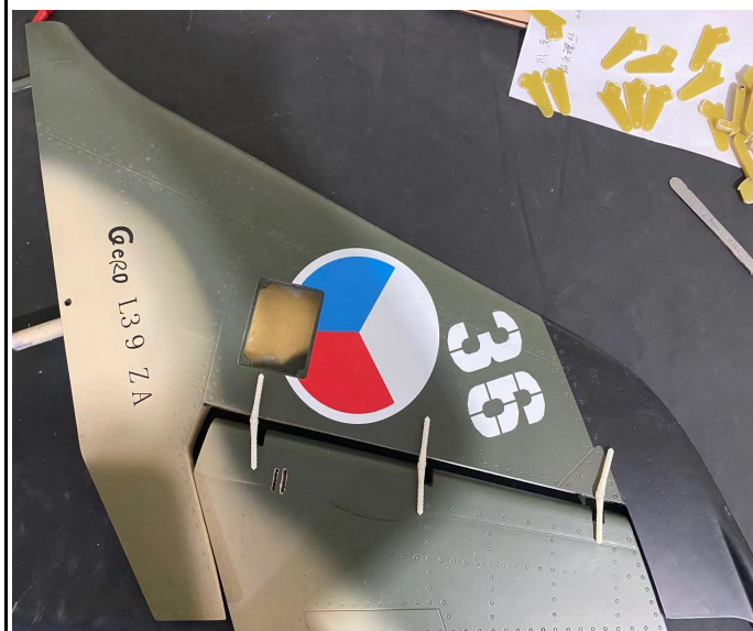
13 Connect rudder with round hinge
