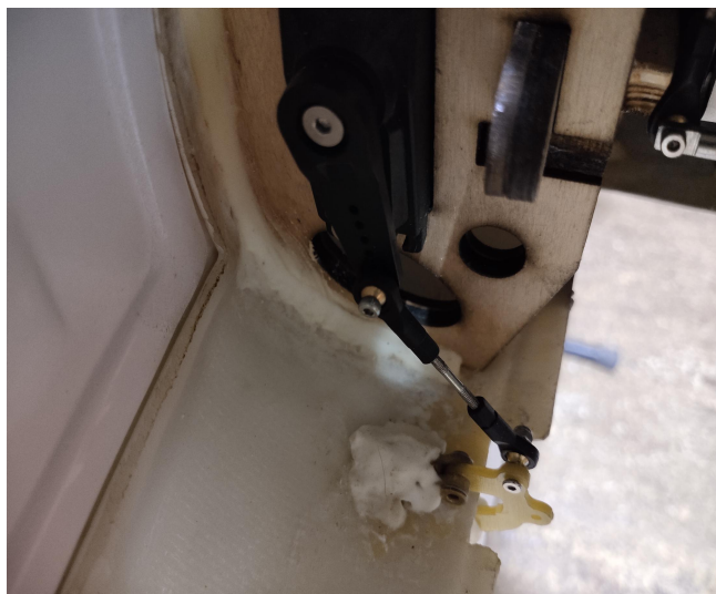
26 connect servo with the front gear door via push rob
