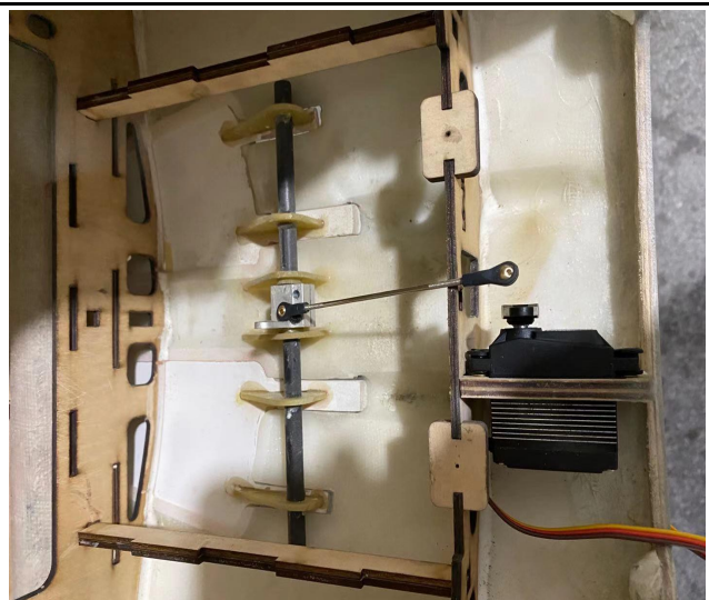
20 Connect the servo and parts of the braking vane via push rob
