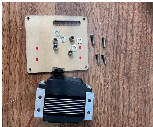
11.Before assemble the servos in stabilizer. Trim slot at proper position
