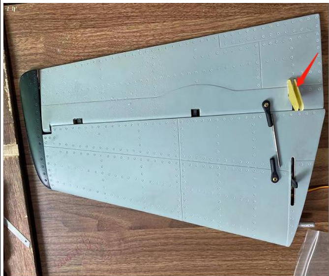
8.Plug the horn in the slot of elevator
