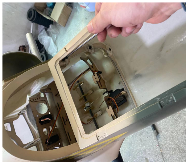
22 fix the front fuselage with screw
