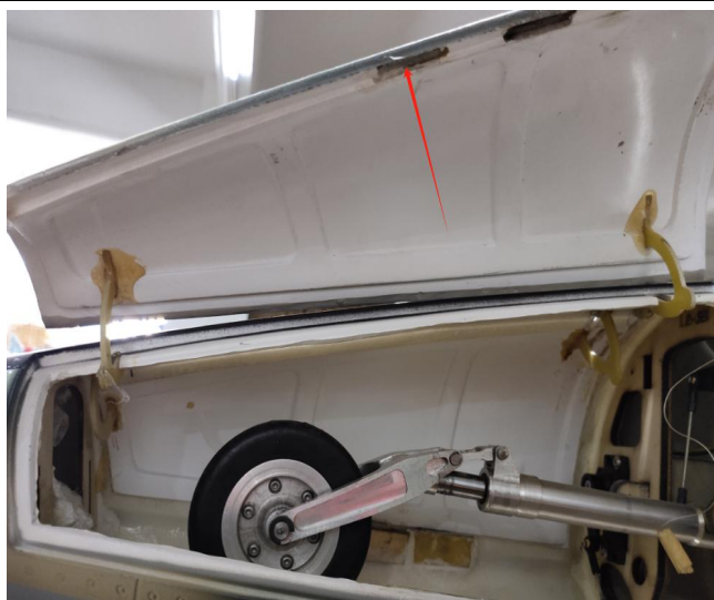
29 The door had magnet for fixing door and front fuselage
