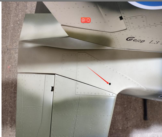
19 Lock the elevator via the hole
