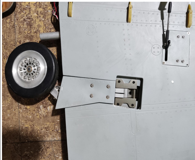
7.Fix retract cover with screws
