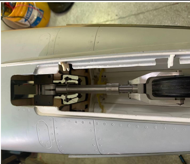
24 fix the front gear on the front fuselage with screw.
