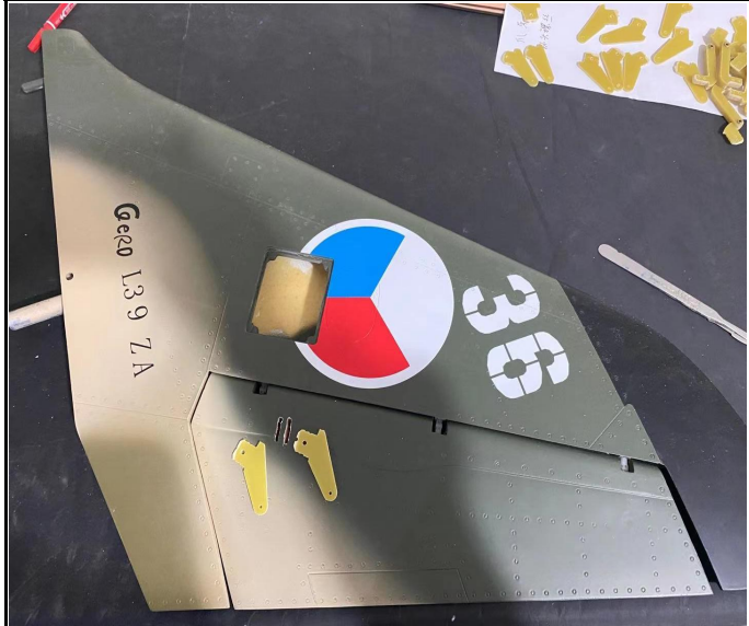
14 Plug the horn in the slot of rudder
