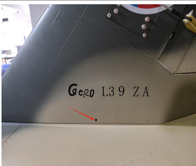
17 Lock the rudder via the hole
