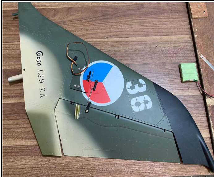
15 Assemble the clevis to the push rod .
